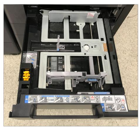
Both length and width guides slide in sync when adjusting paper size in the drawers and have blue locking tabs for easy view. The drawers also feature easy-to-see limit indicators for standard paper, envelopes, and small sizes. The soft close drawers make for no slamming of cassettes, and also pull our far enough for easy access in case of misfeed.
