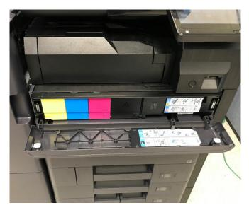
The process for replacing toner is simple and clean. Only when the container is empty will the device notify the user to open the front panel and make the replacement, helping to prevent premature replacement of toner. Guidance at the control panel is extensive and includes text, graphics, animation, and video.
