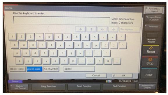
The electronic QWERTY keypad appears when a search key is selected, or when entering an email destination from the scan screen. The keypad is large, and the keys are comfortably spaced. Dedicated "@" and "." Keys are provided on the main screen, but the ability to store extensions (.com, .net) is not supported, nor are typical domains (@gmail.com, @yahoo.com). A subject and three body templates can be stored. A hard keyboard is available as an option.
